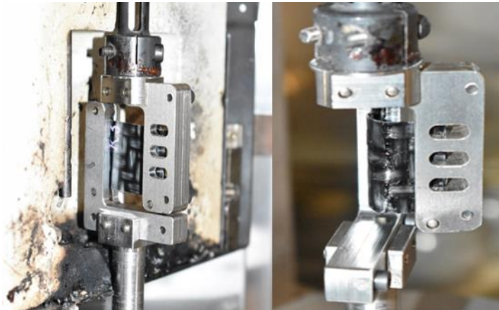
Development and testing of the bending fixture
