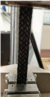
d: Shear Test ISO 14129: 1997
