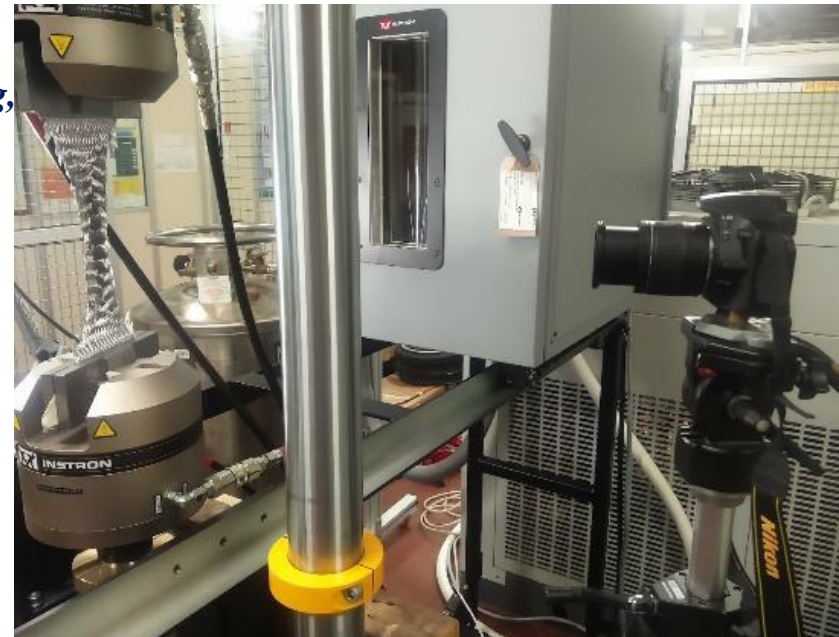
Bias extension test setup
