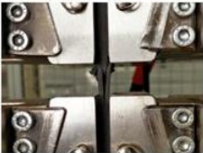
b: Compression Test ISO14126:1999
